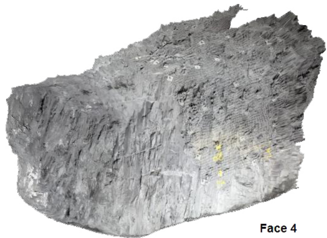
FIG 5 – Photogrammetry pickup of revised perimeter charge.
