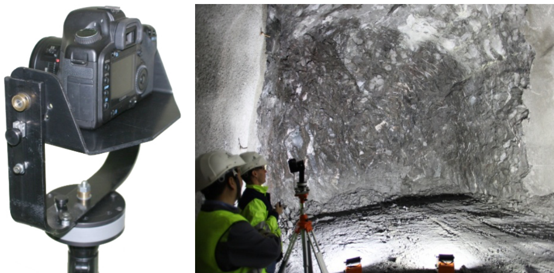
FIG 1 – Camera/mount and underground field kit in operation (images courtesy of Adam Technology).
