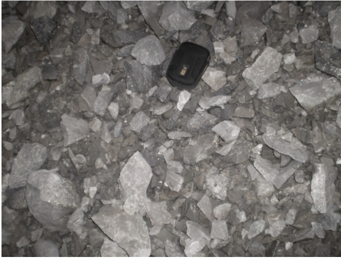
FIG 9 – Fragmentation and butt identification.
